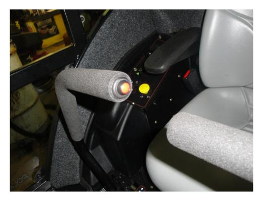
Figure 2 – Push button harness installed and foam grip cut
