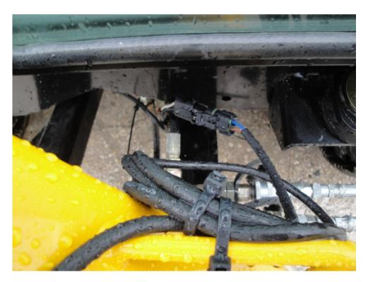
Figure 3 – Adapter Harness Connected to Attachment Harness
