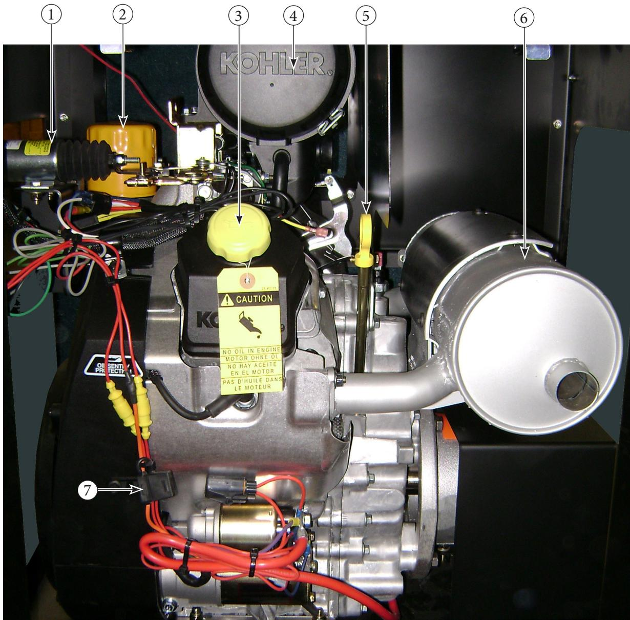
1. Engine Throttle & Choke Solenoids (2)
