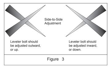
Broom head may be either pitched down too far forward or up too far backward on either side swing arm, giving us the impression of a bowtie. The swing frame bolts must be adjusted either out or in, either separately or together, to achieve a balanced pattern. See Figure 4.
