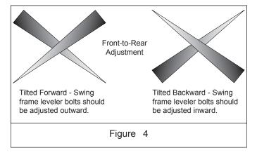
Once the broom has been properly adjusted, a short operation period is recommended for break-in; approximately 15 minutes. After this break-in period, repeat the leveling procedure to ensure that it is correct.
