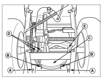
Figure 18. Broom Pulley Belt Stops (shown with bottom cover removed)
