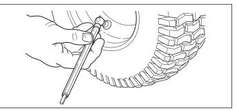
Figure 8. Checking Tire Pressure
