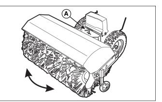
Figure 3. Brush Angle Adjustment A. T-nut
