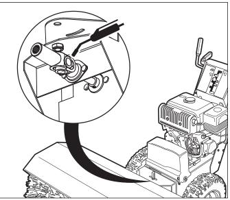
Figure 12. Grease Universal Joint
