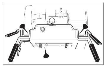
Figure 9. Lubricate Free Hand Control Linkage
