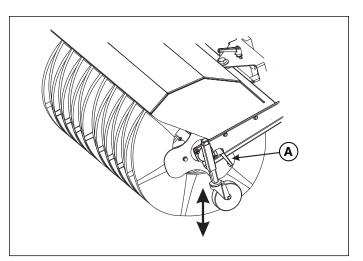
Figure 5. Caster Adjustment A. Caster wheel lock lever
