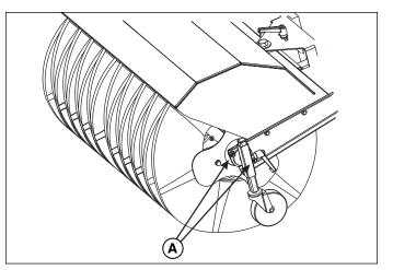
Figure 20. Brush Removal A. Attachment bolts
