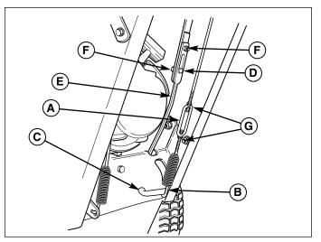
Figure 13. Speed Selector and Broom Drive Linkages
