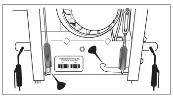
Figure 11. Grease Axles and Control Levers
