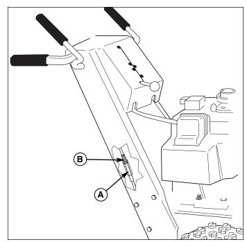
Figure 15. Cable Adjustment A. Adjustment Nut B. Jam Nut
