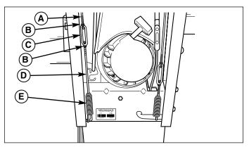
Figure 14. Drive Tension Adjustment A. Upper Rod
