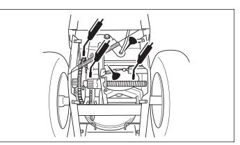
Figure 10. Drive Lubrication
