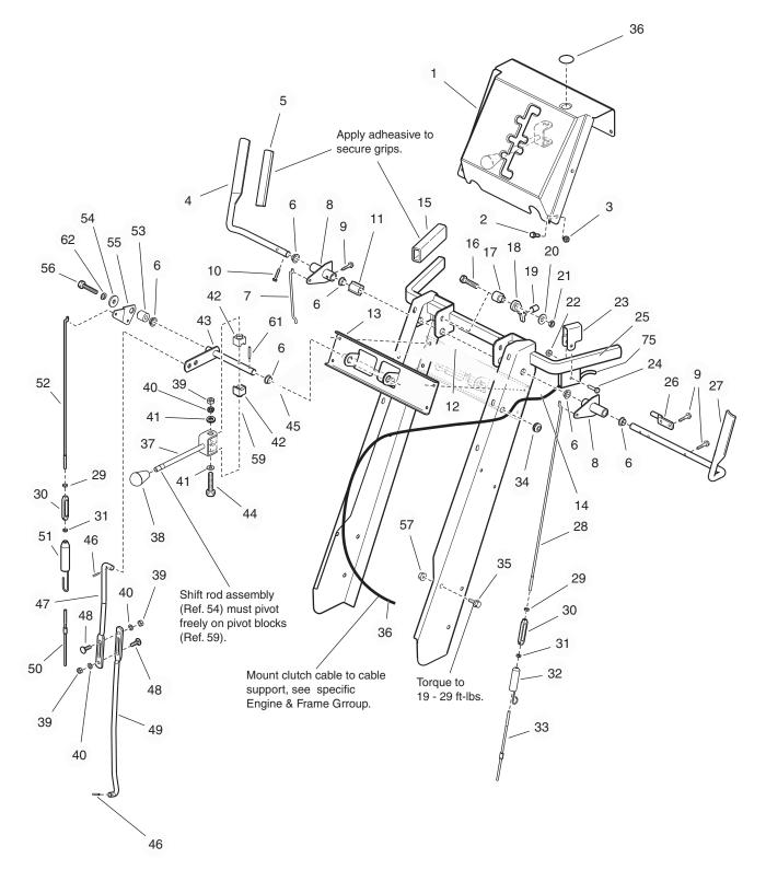
Linkage adjustment for traction and broom drive with power boost: with drive levers engaged, the bottom end of lower rods (Ref. 33 & 50) should be flush with bottom of springs (Ref. 32 & 46).
