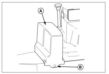
Figure 16. Belt Cover A. Belt Cover B. Screws
